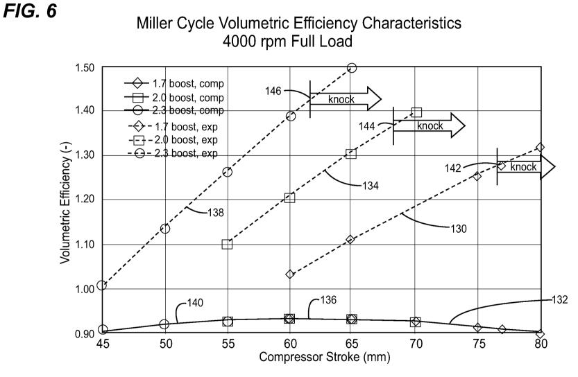
Vol-Eff for comp. cylinder referenced to intake manifold. Vol\_Eff for exp. cylinder referenced to ambient
