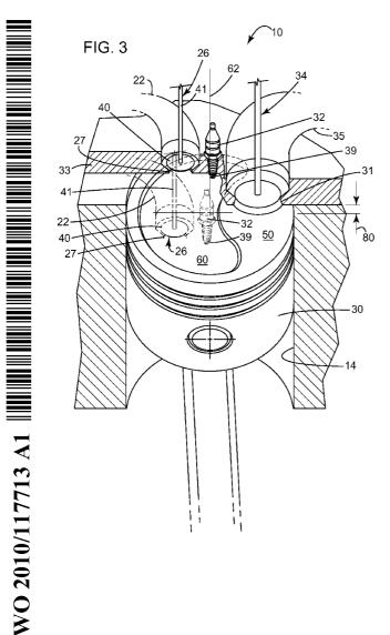
(57) Abstract: The present invention provides a recess in the top (or crown) of the expansion piston of a split-cycle engine for improving the distribution of fuel in the expansion/power cylinder and improving the air/fuel ratios over the spark plugs.
